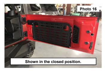
13. Use the latch on each side of the tailgate table to secure the table in the closed position. See Photo 17.
