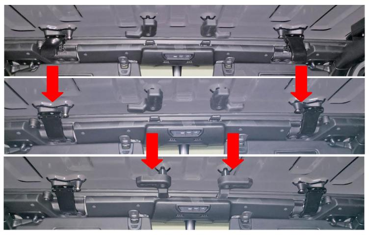
4. Close the rear two L-shaped clamps. (picture pointing to the rear clamps)
