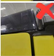
Important note: Ensure that the factory weather seal on Jeep is sticking out just like it was from the factory freedom panels. Trying to hide the seal by pushing it under the top can compromise the weather-tightness of your Jeep, potentially allowing moisture or other elements to enter. To avoid this issue, make sure the weather seal is properly installed and sticking out as it should be.
