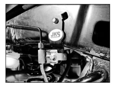
Cycle the suspension to full droop to ensure the brake lines have enough slack and clearance to the sway bar.
