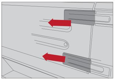
6. Attach HD Hinge Casting to corner panel using supplied 5/16" hardware.
