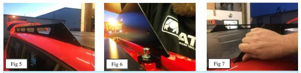
Now, place the side rails into position with logo at rear of vehicle (see fig 5) and install the M6 x 10MM socket head hardware to attach the rails to the roof (see fig 6) *(leave rails loose at this time)* Now repeat on the other side. Next, slide both rails as far back as possible and tighten the hardware. *(some hardware is hard to get to once the front panel is installed)*
