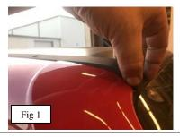
Begin by removing the molding from the roof (both sides). You will need to start from the front edge using a small flat blade screwdriver to get under the molding and lift up to remove.
