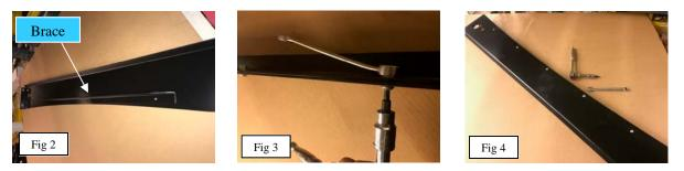
Next, locate the front panel and brace (see fig 2) line up the holes and assemble using supplied M6 x 12MM button head hardware. (*Note: the bolt head should be on the front (See Fig 4*).
