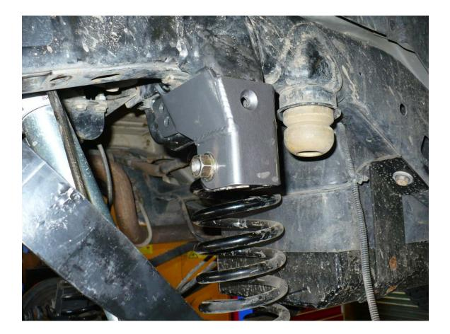
4) Start the 2 7/16" bolts and ½" bolt as shown in the pictures below. Do not tighten yet. Simply start bolts and nuts to align bracket.
