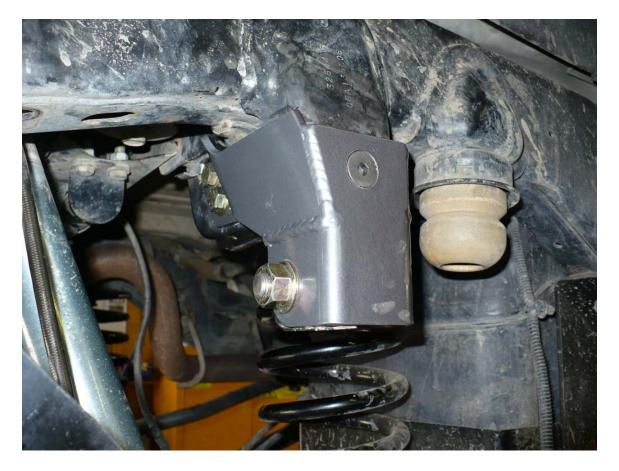
9) Reinstall rear tire and lower vehicle to the ground. Connect TB and new TB bolt and torque to 110 ft-lbs.
