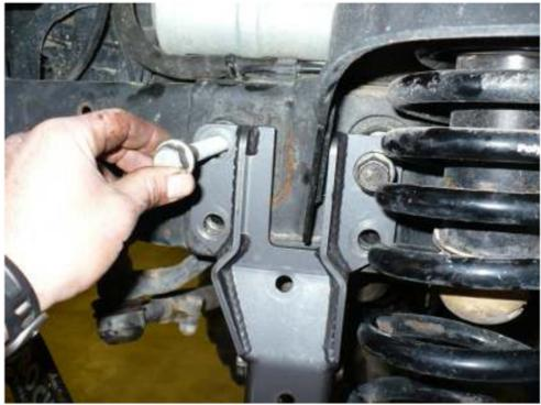
Install the two 7/16" bolts with washers under the bolt and under the top lock nuts on the inside of the bracket
