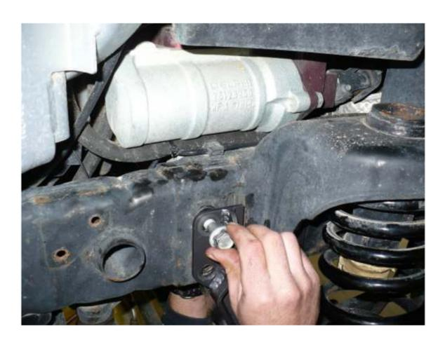
4) Next, install the PPM-8069 Track Bar Brace by fitting it over the factory track bar mount and installing the M14 x 1.5 bolt provided in the kit. (Note: do not install the nut at this time, the bolt is just to hold the bracket in place for the time being.)
