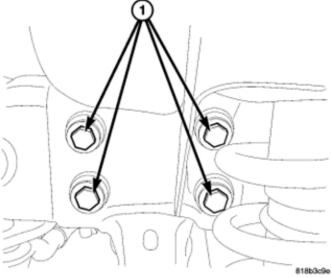
Torque the 2 7/16" bolts installed in step 6 to 70 ft-lbs
