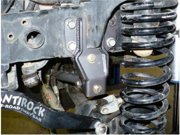
Torque the 4 steering box bolts (1) to 70 ft-lbs
