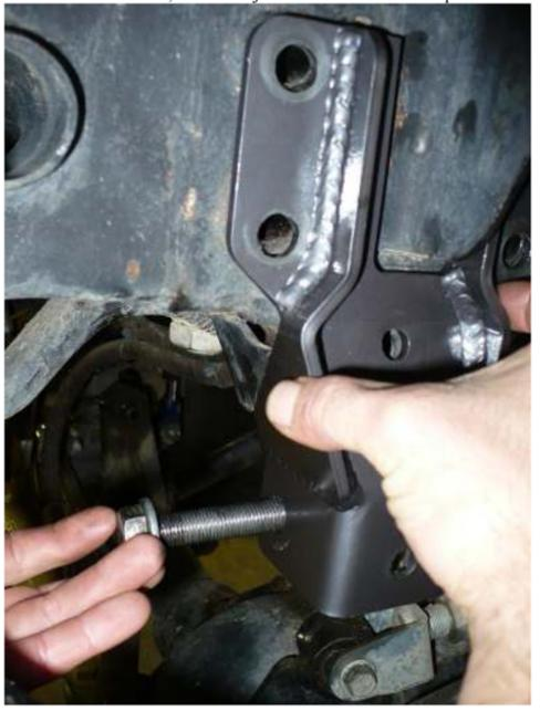
5) Next, align the holes in the steering box with the holes on the bracket and the holes on the frame and loosely install all 4 steering box bolts removed in step 3.
