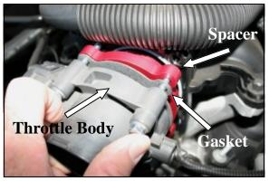
3. Install the Poweraid Spacer and the fiber gasket between the intake manifold, and the throttle body, as shown. Tighten all 4 throttle body bolts evenly, to the manufacturer's specifications.
