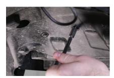
**4.** Remove the two 8mm bolts and one 10mm bolt holding the fender liner in place.
