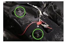
**5.** Pull the fender liner back to gain access to the DRL/sidemarker bracket. Remove the three T27 bolts and loosen the two 10mm bolts holding the bracket in place.
