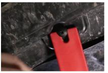
**3.** Remove the Philips head rivet directly underneath the DRL using a plastic trim removal tool.
