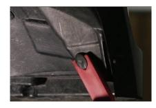
**1.** Remove the four tree clips holding the fender liner in place inside the wheel well using a plastic trim removal tool.
