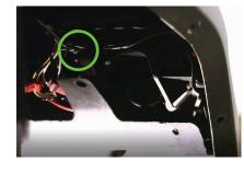
**7.** Disconnect the factory sidemarker wiring harness. To do so, use a pick tool to gently separate the connectors.
