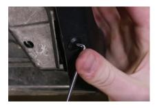
**2.** Using a pick tool, remove the push rivet near the sidemarker on the side of the vehicle. Insert the pick tool into the center of the push rivet and apply pressure to release it. Then using the pick tool, pull the rivet out.
