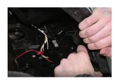
**6.** To gain access to the sidemarker, pull back on the fender liner and pull the DRL bracket down and out to release it.
