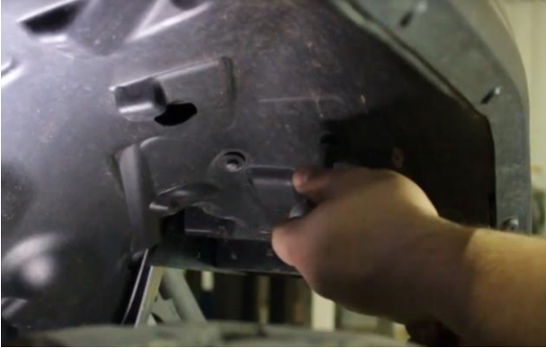
Remove the 2 bolts with an 8mm Socket and the retainer clip.
