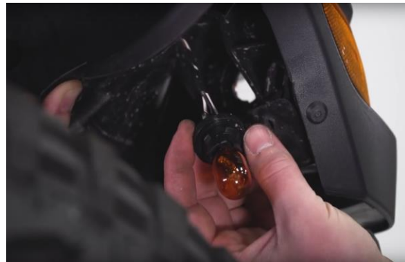
Pull back the inner fender liner and turn the turn signal socket connection counterclockwise to pull away from the housing
