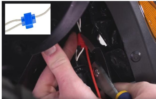
insert the RED grill harness wire into the clip and clamp.
