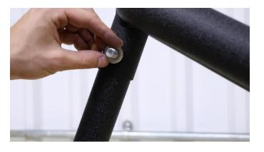
With the hub mount and frame, secure the two with 4 M12 bolts, 4 M12 washers, 4 oversized washers, 4 Nyloc nuts, and 2 19mm sockets.
