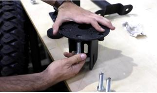
Begin loosely assembling the hub mount. With three of the M12 bolts, 3 washers, 3 oversized washers, 3 Nyloc nuts, and 2 19mm sockets or wrenches, assemble the hub loose enough so that you are able to pull and push the part to the correct mount size.
