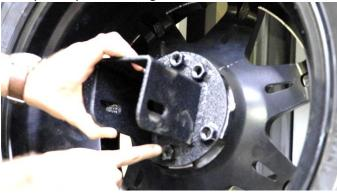
With the 3 M14 bolts and a 21mm wrench, screw them into the upper mount with thread locker so that they match your lug's pattern.
