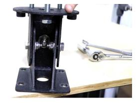
Hold the mount up to your tire and adjust its length so that the mounting plate is flush or near flush with the tire, ensuring that it will lie properly on the mount.
