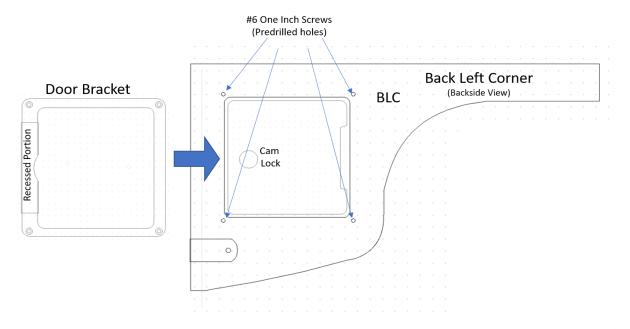
\*Tip: Install the Cam Lock with the 7/8" Wrench. Ensure the lock is oriented with the cut portion of the key in the up facing, or down facing position, whichever is preferred. Place the Inner Retaining Ring with
