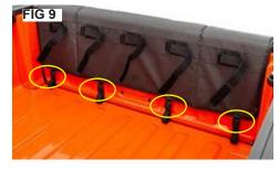
Repeat this procedure for the two outside straps. (Fig's 7 & 8). Tighten and secure all four of the straps (FIG 9-Circled). Adjust the pad by rotating it or pulling it in the direction needed so the front facing safety straps are positioned as shown in FIG 9.
