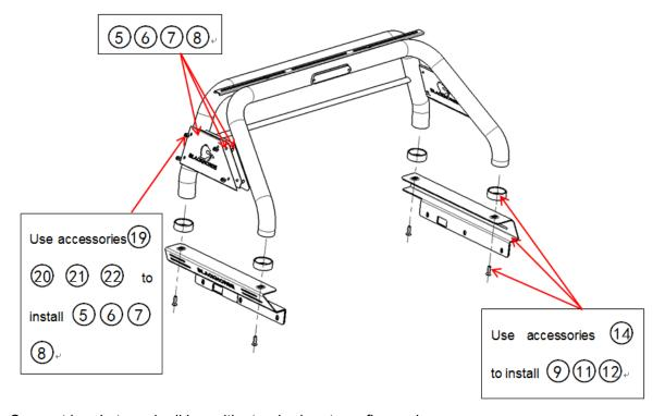
**Step 3:** Connect brackets and roll bar with standard parts as figure shows.
