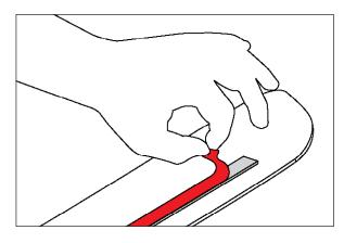
5. Attach rocker guard to the vehicle keeping part aligned to the vehicle surface. Apply pressure to ensure a strong bond. Tighten bolts and nuts.
