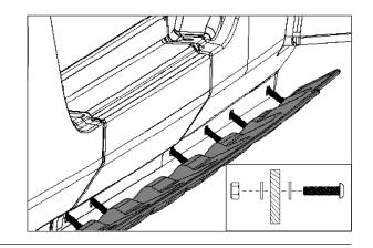
4. Peel red liner from back of tape working from outer edges inward. Make sure that all tape covering is pulled back at the same time. This will insure that all the protecitve covering is removed during installation.
