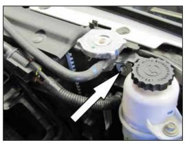
10. Remove the bolt show that secures the radiator to the core support.
