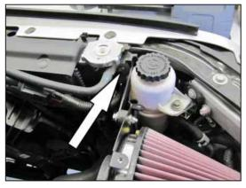
19. Install the heat shield bracket assembly onto the heat shield and radiator mount as shown. Secure the bracket with the factory bolt in step # 9 and the hardware provided.
