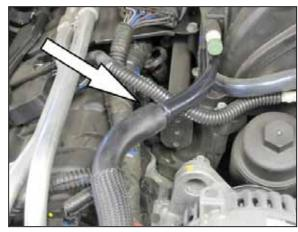
7. Disconnect the crank case vent hose from the crank case vent tube
