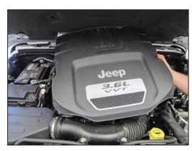
2. Lift up and remove the engine cover.
