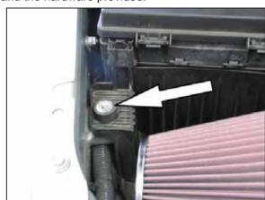
20. Install the rubber mounted stud into the into the air box mounting plate bolt location as shown.
