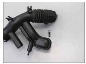
27. Remove the inlet air temperature sensor from the factory intake plenum as shown.
