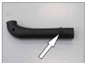
25. Install the 90 $^{\circ}$ ,  $\frac{1}{2}$ " vent fitting into the K&N intake tube as shown.
