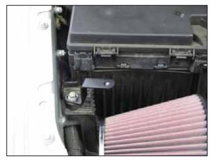
21. Install the provided bracket (083163) onto the rubber mounted stud using the provided hardware.
