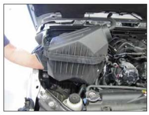
8. Lift up and remove the air filter housing from the vehicle.
