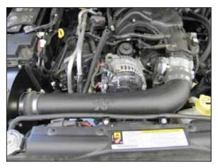
31. Install the K&N intake tube into the silicone hose at the filter adapter and then into the hose at the throttle body, then secure with the provided hose clamps.
