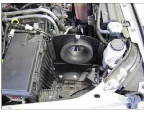
16. Install the heat shield assembly into position so the mounting studs are in the air box mounting arommets.
