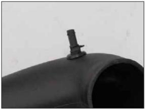
28.Install the provided grommet and factory inlet air temperature sensor into the K&N intake tube as shown. NOTE: Be sure to remove the O-ring from the sensor before installing it into the grommet.
