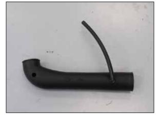
26. Install the provided crank case vent hose onto the fitting as shown.
