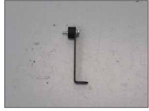
18. Install the provided rubber mounted stud onto the heat shield bracket (083164) as shown.
