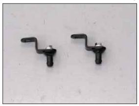
11. Install the two provided mounting studs onto the two heat shield brackets (070061) as shown
