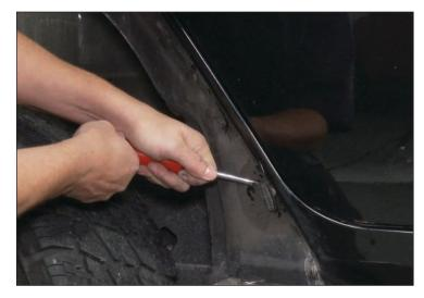
5. The fender is attached to the body using nutserts. There are available at most automotive tool stores or online. We recommend using the tool shown here.
