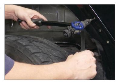
6. To install the nutsert, load tool properly with a nutsert. We recommend applying a small amount of RTV silicone to the edge of the hole to fully seal the nutsert to the body and to avoid water or debris to enter. Insert nutset into the body of the Jeep and crimp. Take your time crimping to assure it's fully crimped. This will avoid the nutsert from spinning or being crooked.
