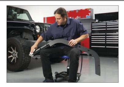
2. When applying the fender seal, peel back a small portion and apply to the fender. Peel and press along the entire top edge of the fender. Once you reach the bottom rear edge of the fender trim seal with a scissors of utility blade.
