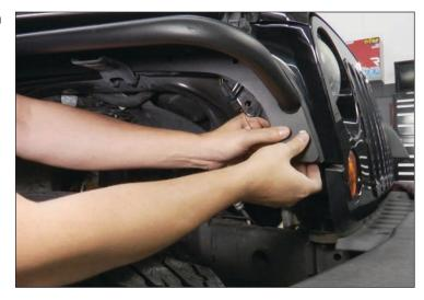
8. Use a 12mm and 14mm open end wrench to tighten hardware. Must use a open ended wrench due to the tight space between the OE sheet metal. Tighten all hardware in a alternating pattern.
