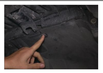
2. Remove body clips that attach the inner fender to the body. Use special removal tool or flat head screwdriver to pry out.
