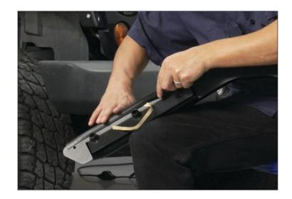
3. The entire rear fender and liner is attached with body clips. Pull and/or pry the inner fender clips away from the body first. Now the inner fender is free left up and out to pull the fender away from the body.
