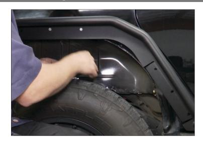
8. Now tread the bolts into the remaining nutserts. Avoid using power or air tools, now tighten all hardware with hand tools in a alternating pattern. That completes the install of your steel tube fenders.
