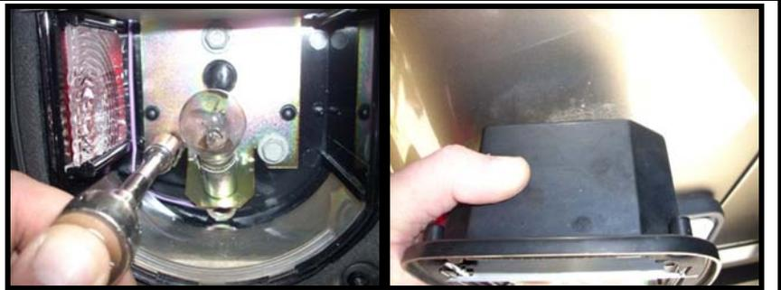
**Step 5:** Carefully pull the tail light wiring through the hole. Guide the connector through the hole.
