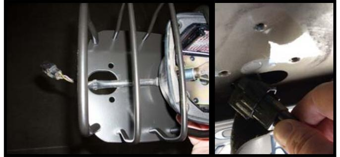
**Step 9:** Reinstall the tail light assembly and Euro Tail Light Guard to the original mounting holes using the new bolts provided.
