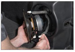
Remove the grill and factory subwoofer. Disconnect the two connectors from the woofer.
