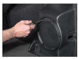
Using a T20 torx driver remove the 6 screws from the factory subwoofer grill.
