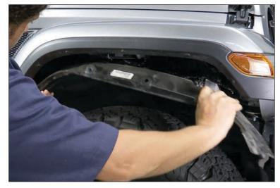
2. Remove the lower fender brace located at the rear bottom of the fender.
