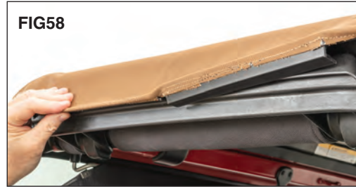
Starting with the front strips, slip the strips into the channel in the door surround
