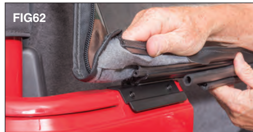
Open the rear tailgate. As shown in FIG62, insert/roll the tailgate bar into the mounts on each side of the tailgate with the vinyl side of the rear curtain facing the rear of the vehicle.
