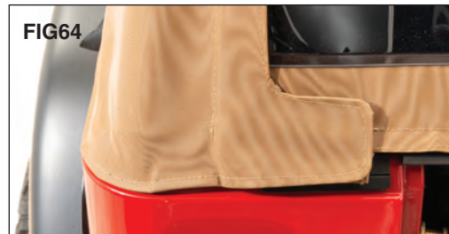
(FIG63) and then secure the rear zipper cover flap as shown in FIG64.
