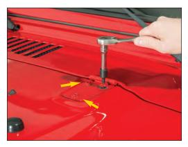
Torx bit and ratchet. (it may be necessary to score the paint around the bolts using and razor blade to prevent paint chipping.)
