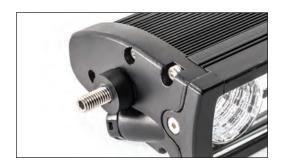
On the Passenger side of the light bar, install one of the M8 studs (supplied with Ouadratec light bar) using a 4mm hex key. Also install one of the supplied spacers on the stud.
