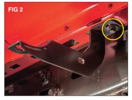
Align the hole in the step mounting bracket (PF) and loosely install using a 8 x 35mm bolt (B), lock washer (J) and flat washer (H). (FIG 2)
