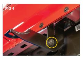
Next align the mounting slots between the two brackets and loosely install a 10mm bolt (A) with washers (G) on both sides and secure with a 10mm nylock nut (E) using a 16mm hex wrench and a 17mm socket. (FIG 4)
