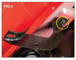
Align the hole in the step mounting bracket (PM) and loosely install using a  $8 \times 35$ mm bolt (B), lock washer (J) and flat washer (H). (FIG 6)
