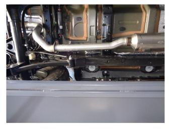
**Step 2:** With the system supported, working front to rear disengage the hangers from rubber insulators and remove the OEM system. Do not discard or damage the clamp or rubber insulators as they will be used to install the new system.
