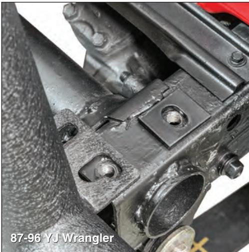
*If you are installing the winch plate on a YJ Wrangler with a Tube style bumper place the supplied spacer plates over the 2nd mounting holes in your frame as shown above. Repeat for other side.*
