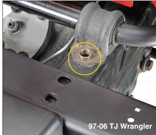
*For use with a stock TJ bumper, place the supplied spacer rings over the sway bar bolt holes on both sides.*
