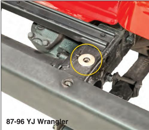
*When installing winch plate on a YJ with a stock bumper place a supplied 1/2" washer over second bumper hole.*
