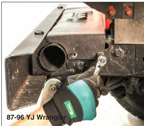
Put on safety glasses. Remove frame / sway bar cover by removing the 2 bolts on either side with a 3/8" socket.
