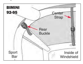
SECURE REAR CORNER STRAPS **For Bimini:** (see above) Locate the straps sewn near the rear corners of the Bimini. Wrap them under the sport bar, through the loop, under the rear sport bar and thread the end of each strap through the buckle. Do this on both sides of the vehicle. Then pull the straps tight through the loops as well as the buckles.
