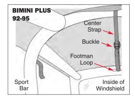
man loop located above windshield. Pull the end of the strap back and thread it through the buckle (see diagram above) on the strap. For Bimini, pull strap tight at this time. For Bimini Plus: Do NOT pull the strap tight at this time.
