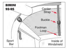
INSTALL TOP TO ROLLBAR Locate the long web strap sewn to the center flap inside the top. Wrap the strap around the horizontal tube of the sport bar and pull it toward the front of the vehicle. Thread it through the foot-
