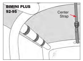
For Bimini Plus: (see above) Locate the three pairs of hook & loop strips sewn to each side of the top, above the door opening. Wrap the strips around the sport bar and fasten them to each other. Make sure that all the hook and loop is as tight as possible. Continue to final step...
