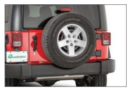
Close the tailgate and reinstall the spare tire and secure it with the 3 lug nuts. Tighten by hand and do not use an impact gun. This could overtighten the lug nuts and damage the 3rd brake light ring.
