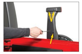
Open the tailgate of the vehicle and locate the 4 T20 screws on the backside of the factory 3rd brake light housing. Remove the 4 screws with a T20 torx driver.
