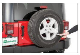
Put on safety glasses. Remove the lug nuts that secure the spare tire using lug wrench and correct socket (factory lug nuts use ¾" socket). Carefully remove
