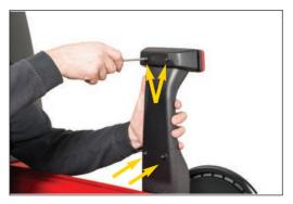
Reinstall the factory brake light into the tire carrier housing. Be careful not to pinch any of the wires while reinstalling. Reinstall the 4 T20 screws with a Torx driver.
