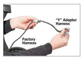
Plug the supplied "Y" harness into the factory harness as shown. Make sure the connectors fully engage & lock together.
