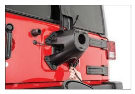
the spare tire. Pass the connector and harness from the third brake light ring behind the spare tire carrier and out the top.
