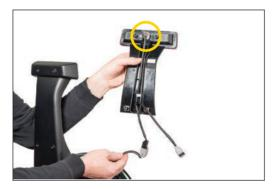
Now plug one end of the "Y" harness into the back of the factory brake light. Once again make sure the connectors fully engage and lock together.
