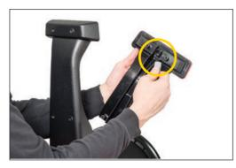
Remove factory brake light from the housing and unplug the factory connector from the back of the brake light.
