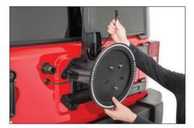
Place the third brake light ring over the studs on the tire carrier as shown with the attached harness located at the bottom of the ring. You may temporary secure the brake light ring by finger tightening one of the lug nuts on to the tire carrier studs.
