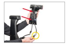
Route and secure the "Y" harness into the channel on the backside of the brake light. Use the same routing and securing clips that the factory harness used. Connect the other end of the "Y" harness to the brake light ring harness.
