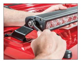
While supporting the light bar pass the stud through the hole on the Passenger side hood bracket and secure it with a washer, split washer, and nut. Tighten using a 13mm wrench.
