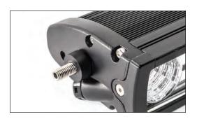
On the Passenger side of the light bar, install one of the M8 studs (supplied with Quadratec light bar) using a 4mm hex key. Also install one of the supplied spacers on the stud.
