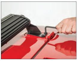
Fully tighten the hood fasteners at this point with a T40 key.
