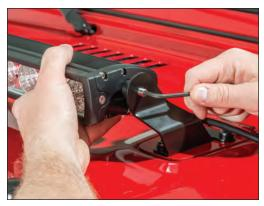
Install the spacer between the bracket and lightbar and install stud through the bracket using a 4mm hex key. Install the washer, split washer and nut and tighten with the 13mm wrench as shown above left.
