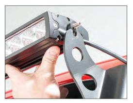
Drop the stud on the driver's side down into the slot.
