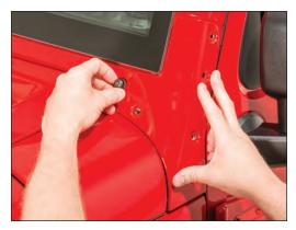
and ratchet. Retain bolts for reassembly and be careful not to drop the hinge plate after the bolts are removed.
