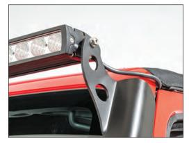
Install washer, split washer, and nut (supplied with lightbar) on both sides.
