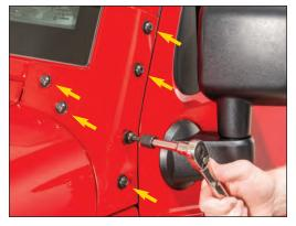
Put on Safety Glasses. Locate the 6 T40 torx bolts on both windshield hinges. Remove all 6 bolts using a T40 Torx bit
