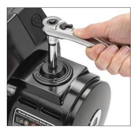
Once the Clutch Handle is removed, it can be stored in the vehicles glove box or console and used only when winching.
