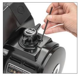
Rotate Clutch Handle to the "FREE SPOOL" position to reveal the set screw that holds the handle in place. Using a 2.5 MM Allen wrench, back out the set screw until the Clutch Handle lifts off but do not remove the handle at this time.
