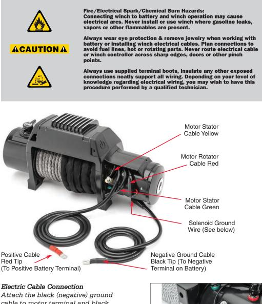
cable to motor terminal and black solenoid ground wire with brass bolt. Tighten the brass bolt onto terminal using a 13mm wrench. Then attach positive and negative cables to their corresponding battery terminals.
