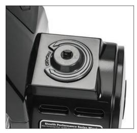
Rotate the clutch selector to the "EN-GAGED" position. You may remove the Clutch Handle now and keep it in a safe place. We suggest keeping the Clutch Handle somewhere in the vehicle,
