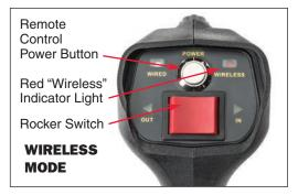
light will remain lit while it is connected to the winch. If the red light on the controller begins blinking while operating the winch, the controller is out of range. Move the controller closer to the winch until the light stops blinking. Test both the "OUT" and "IN" functions of the winch using the rocker switch. The winch is now ready for use.
