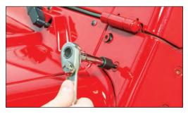
Install driver side bracket as shown with the supplied 5/16 T40 head bolts and nylon washers.
