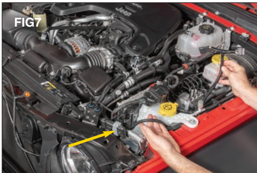
Route the harness behind the headlight and past the reservoir bottle towards the firewall on the drivers side.
