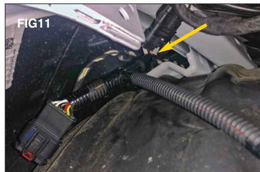
the OEM harness until you hear a click and then push the red and gray locking tabs to lock the connections. (FIG 11)
