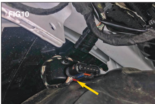
Slide the red locking tab backwards and disconnect the plug. (FIG 2) Then, plug in the new Tee harness to each side of
