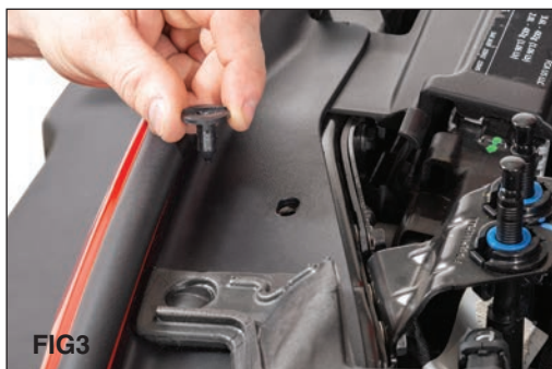
Pry up the plastic fasteners (6 total) using a small flat blade screwdriver. First remove the center, then remove the body of each plastic retainer (FIG 3). Set rivets aside in a safe place for re-installing the grille.
