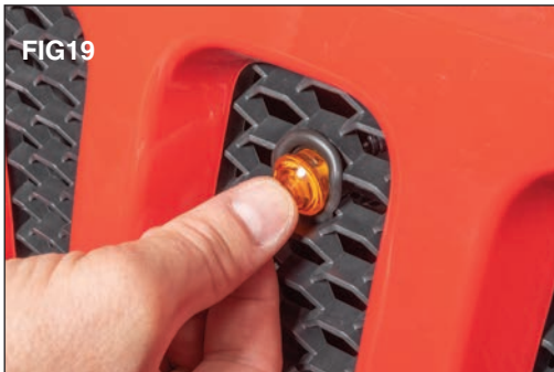
Push the LED light into the grommet to seat the light into the grill insert. (FIG19)
