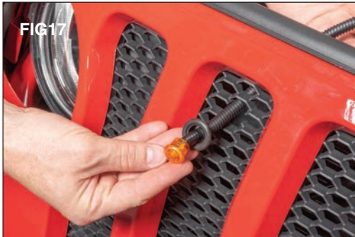
Separate the grommet from the LED light on the harness and pass both the grommet and light through the hole in the 2nd grill slot. (FIG17)
