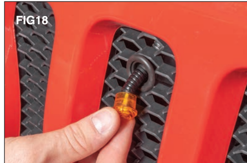
Push the grommet into the hole in the grill insert. (FIG18)
