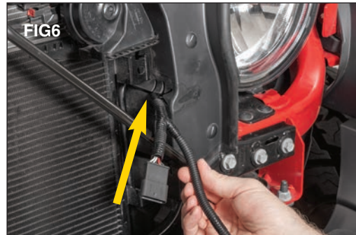
Fish it through the rubber barrier on the driver side of the radiator as shown.
