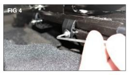
Using a 3mm Hex Allen Key install one M5 x 45mm Screw and Flat Washer in each bracket. (FIG 4)
