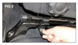
Snap the light bracket to the seat slider as shown. Slide the front bracket as close to the front of the seat as possible. (FIG 2)
