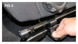
Tighten the M5 x 45mm Screw until the bracket is snug being careful not to over tighten and damage the bracket. (FIG 5)
