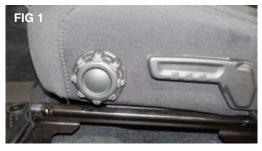
Put on safety glasses. Open the driver or passenger door of your Jeep. Locate the seat slider. (driver side shown) (FIG1)
