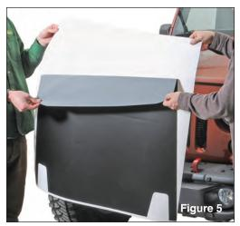
9. With two people, hold the decal vertically so that the end which faces the front of the vehicle is up. Remove the decal from the backing paper.
