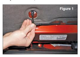
2. As shown in Fig.1, remove the hose(s) from the windshield washer nozzle(s). The hose is simply pressed into place, so just pull it to remove. Remove the nozzle(s) from the hood by pressing on the retaining clips on it's sides, then pushing it up through the hood.
