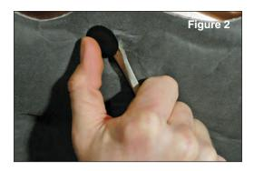
3. Use a flat head screwdriver or a v-notch panel puller to remove the retaining clips (Fig.2) that hold the hood silencer pad in place. The hood silencer pad is the soft material fastened to the underside of the hood.
