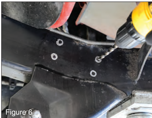
Figure 6 Drill holes in the frame with a drill and 5/16 drill bit. You may want to drill a pilot hole with a smaller bit first. (Figure 6)
