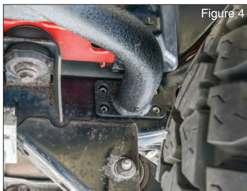
Once the guards have been positioned properly you will need to trace the mounting holes of the front and rear brackets against the frame with a paint pen or marker as shown. (Figure 4)
