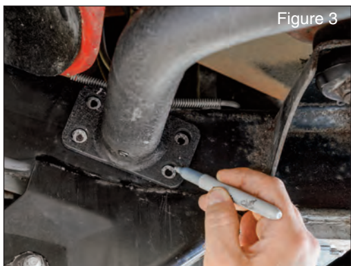
Position the rocker guard so that brackets are positioned flush against the frame in these areas. You may need assistance to ensure that the rock rail or side step is parallel to the body and maintain an even gap of approximately 1 ". (Figure 3)
