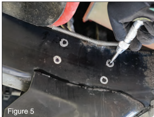
Figure 5 First, put your safety glasses on. Then using a center punch, mark the center of each of the holes. (Figure 5)
