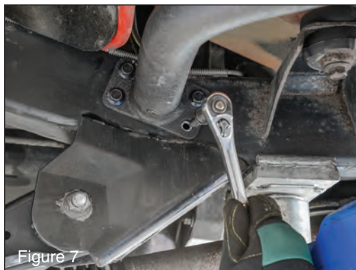
Figure 7 Reposition the rocker guard over top of the holes in the frame and install the (8) 3/8 x 1" self tapping screws with a 13mm socket and ratchet. (Figure 7)
