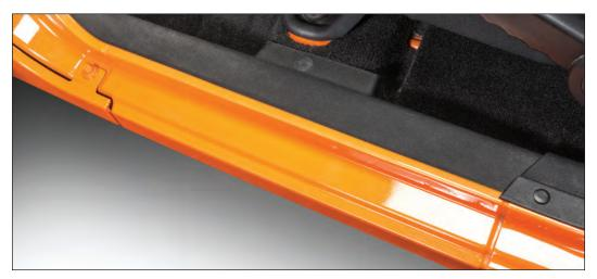
Before You Begin: Put on safety glasses. Remove any existing entry guards along with any prior entry guard adhesives. Thoroughly clean the entire entry guard threshold area with hot soapy water and a clean rag. Dry off sill area with a clean dry towel or chamois. Test fit both
