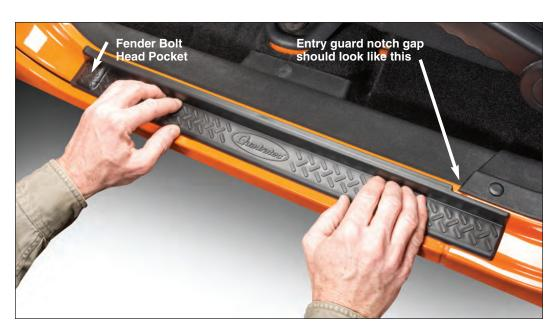
into place. **Carefully** note the proper placement of the entry guard in the photo above. Make sure the entry guard is completely inward as shown. Use
