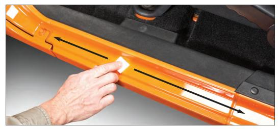
Step 1: Clean threshold contact area with an alcohol prep pad. Remove one alcohol prep pad from its packet and wipe the entire contact area with the
