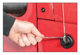
Put on safety glasses. Remove the stock antenna with a 3/8" wrench.
