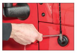
Install the new antenna and tighten gently with a 7/16" wrench.
