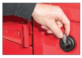
Thread the Antenna Adapter (by hand) into the vehicle antenna mount.
