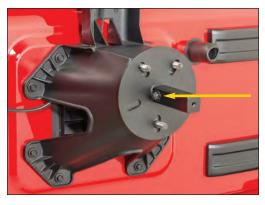
Install the assembled mounting plate and extension on to the spare tire mounting studs as shown. Make sure that the button head bolt on the mounting plate and extension is parallel to the ground.
