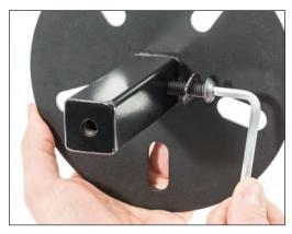
Using a 7/32" hex wrench thread the button head bolt and a flat washer through the extension and into the mounting plate. Snug the bolt with the hex key.
