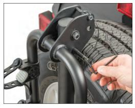
Remove the retention clip and retaining pin from the upper hinge and swing the rack arms into position.
