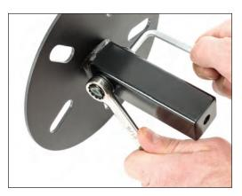
Install a flat washer and nylock nut onto the other end of the bolt and tighten it with a 9/16 wrench while holding the bolt with a hex key.
