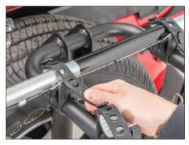
Pull the rubber retaining straps over the frame of the bike and secure it on the rectangular hook.
