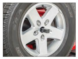
Remove the center cap from your spare tire and remount it on the spare tire carrier so that the Bike rack mounting plate is sandwiched between the spare tire and the tire mount. The Bike rack mounting extension should be protruding through the wheel.
