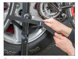
Continue the thread the strap through both wheels and secure it using the buckle.
