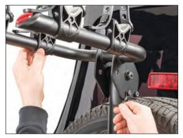
Reinstall the pin and retention clip into the lower hole. Place the bike into the cradles as shown. (The position of the cradles can be adjusted using the provided 5mm hex wrench as shown previously in the assembly portion.)
