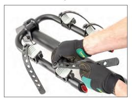
Install the round end of the rubber retaining straps by pulling them over the square retaining tabs on the cradles.
