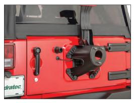
Start by removing the vehicle's spare tire with a ¾" socket and drive or the appropriate lug wrench.
