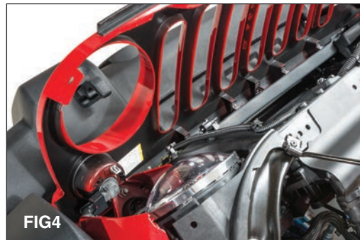
Next, Gently tilt the grille forward and then gently pop the lower portion of grille from its retaining clips. (FIG 4)
