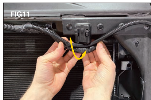
You will need to reach under and pull out the wiring harness to position it in front of the bracket as shown. (FIG 11)
