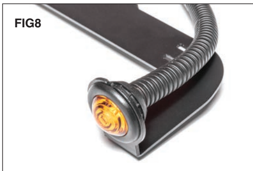
Push the grommet into the mount, push the lamp into the grommet until flush and replace wire loom. (FIG 8)
