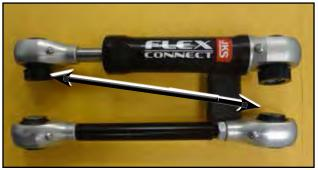
• Adjust the fixed link to be of equal length as the flex connect and lock off the jam nut.
