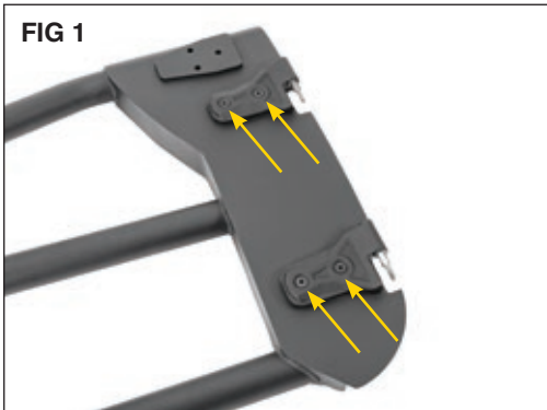
Start by locating the hinge fasteners. Loosen the fasteners on the upper and lower hinges slightly with a 5mm Hex key and a 13mm wrench or socket. (FIG1)
