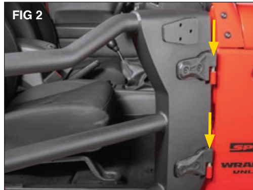
Align the hinge pins with the factory door hinges of your vehicle and gently lower the doors onto the hinges. (FIG2)
