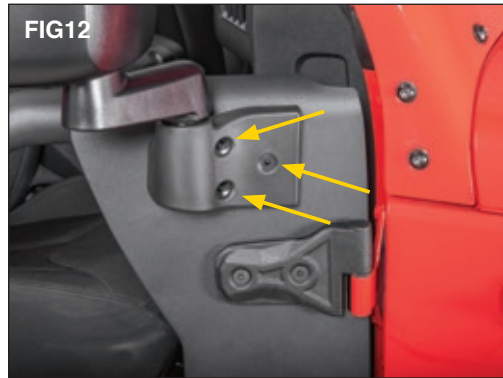
Pass the 1/4" counter sunk screws through the holes in the mirror and secure them with a washer, split washer and hex nut on the inside of the door. Tighten the screws with a 5/32" hex key and 3/8" wrench or socket. (FIG12)
