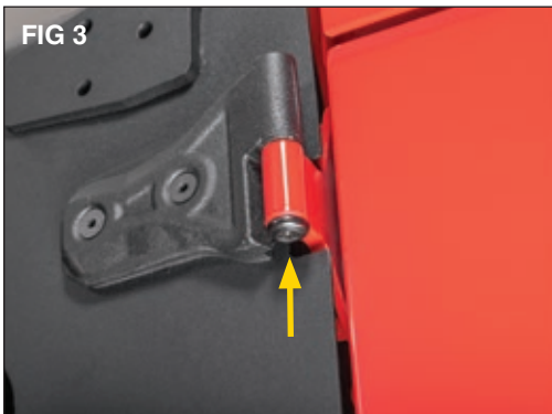
Loosely install the factory door retention nuts with a T50 Torx but do not fully tighten at this time. You may need to wiggle the door in order to align the hinge pins in hinges. (FIG3)
