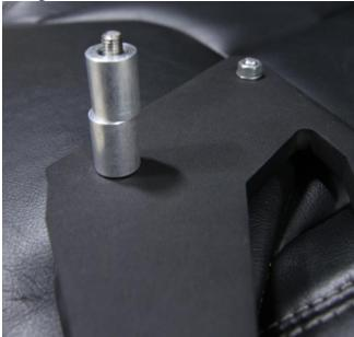
**4.** Next holding the spacers in place so they do not fall off bolt, install bolt into the removed OEM bolt location located in the A pillar. Do not tighten. See image below.
