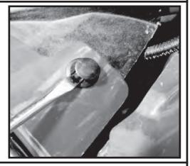
Step 2. Lay the grille with the front side down on a smooth flat surface that will not scratch the paint. A towel or cloth is recommended. Lay the insert onto the back side of the grille matching the same contour. Note that the area that has a small cutout in the insert goes the driver side bottom corner.
