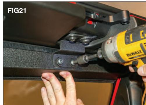
Finally, push up on the light bar and tighten the T-40 screws from bracket to light bar. (FIG 21)
