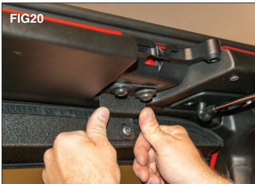
Now push the light brackets forward until they rest against the plastic trim. (FIG 20) You may now tighten the factory T-40 screws. Some adjustment may be necessary to re-align the brackets to your top latches.
