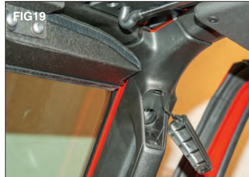
Re-install the grab handle taking care not to pinch any wires. (FIG 19) Also, Re-install the speaker cover.
