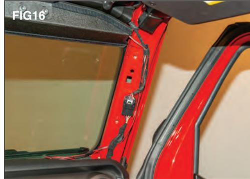
to the brackets using the supplied T-40 torx bolts and washers. Now, route the wiring harness as shown down the A-pillar along side of the factory wiring. (FIG 16)
