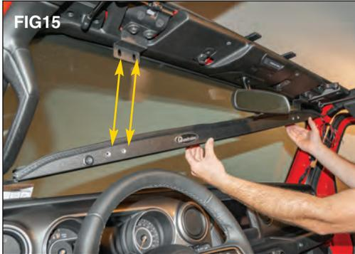
Tilt the light bar into place, careful not to knock off the smaller end gaskets. (FIG 15) Loosely attach the light bar
