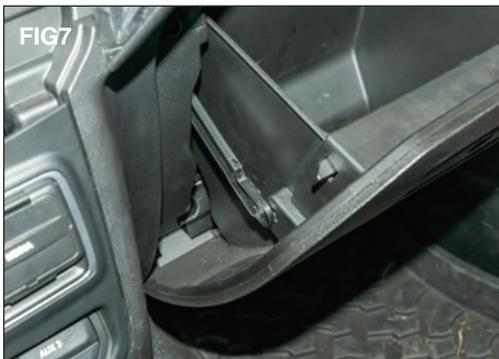
Open the glove box and disconnect the strut on the side by sliding it towards the top of the glove box. (FIG 7)
