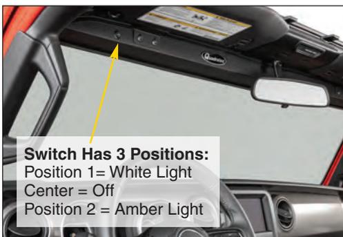
Stealth Light Bar is compatible with the standard rear view mirror as well as the auto-dimming version (above right).
