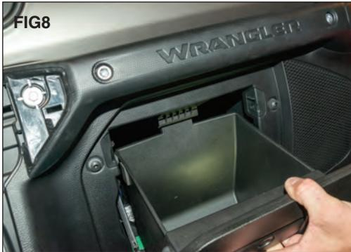
*Push up on the glove box stop, tilt it down, remove glove box and set aside. (FIG8) Now, route the new harness through the dash and out behind the*
