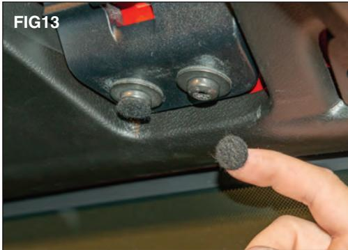
Unlatch and open the soft top or remove hard top front panels. Remove the felt padding on top of the brackets hardware. (FIG 13)
