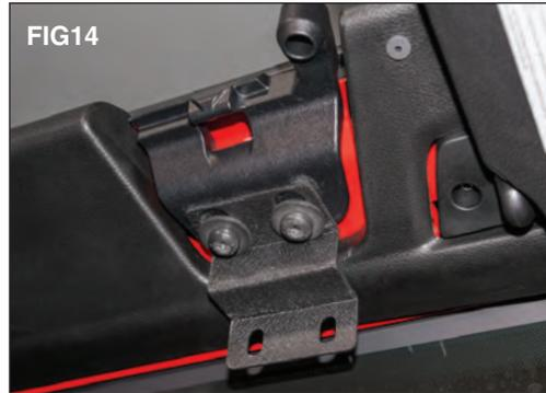
Remove the hardware using a T-40 Torx socket and loosely install the supplied brackets as shown. (FIG 14)
