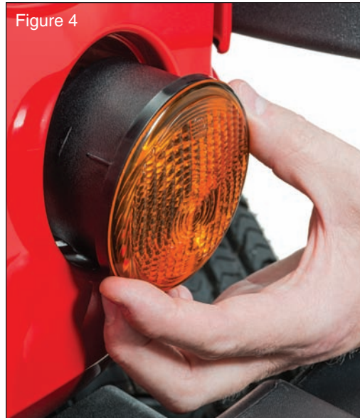
the housing from the grille assembly (Fig 4). The turn signal housing can now be easily removed by pushing it through the grille.
